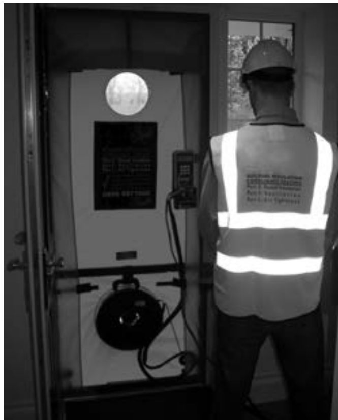
Figure 2.36 Airtightness testing: (a) blower door and (b) trailer fan (reproduced courtesy of BSRIA Compliance)
