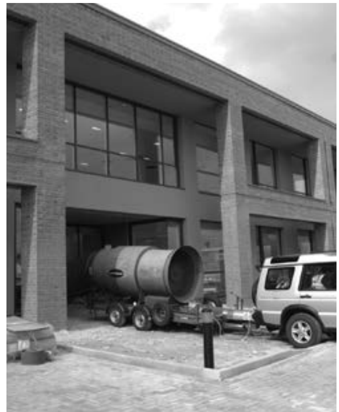
Figure 2.36 Airtightness testing: (a) blower door and (b) trailer fan (reproduced courtesy of BSRIA Compliance)
